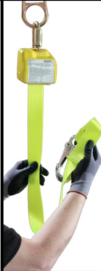
INSPECT LIFELINE FOR DEFECTS
